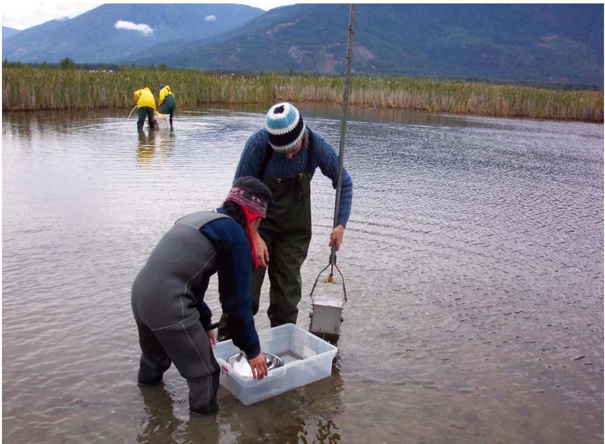
Bed sediment sampling for pesticides at Duck Lake in Kootenay, British Columbia
